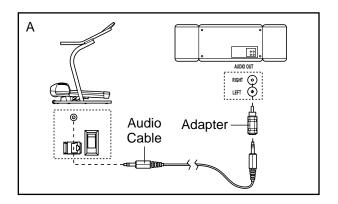
B. Plug one end of the audio cable into the jack on the side of the hiker near the power cord. Plug the other end of the cable into the LINE OUT jack on your stereo.
